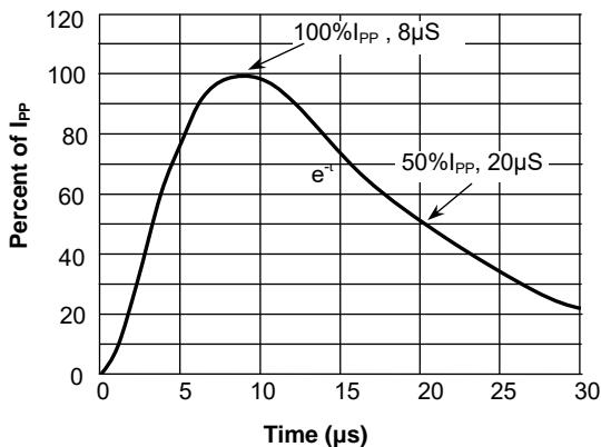
**Fig.4 Pulse Waveform-ESD(IEC61000-4-2)**
